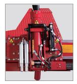
Features a tool carrier trolley attachment system, which ensures the tool carrier arm and trolley are connected securely and safely.
